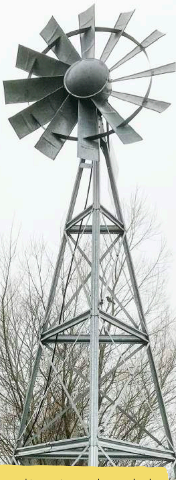
Wind turbine used to aerate a pond on a school ground greening site at Milliken Mills High School in Markham, ON (EcoSpark 2018)
